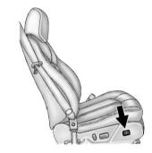
If available, hold the control on the outboard side of the seat forward or rearward to increase or decrease the lumbar support on the driver or front passenger seat.
